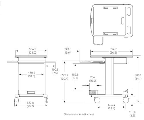
Figure 20. Keysight 1184A testmobile cart dimensions.
