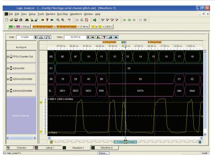
Figure 6. Make time-correlated measurements between an Keysight logic analyzer and oscilloscope.
